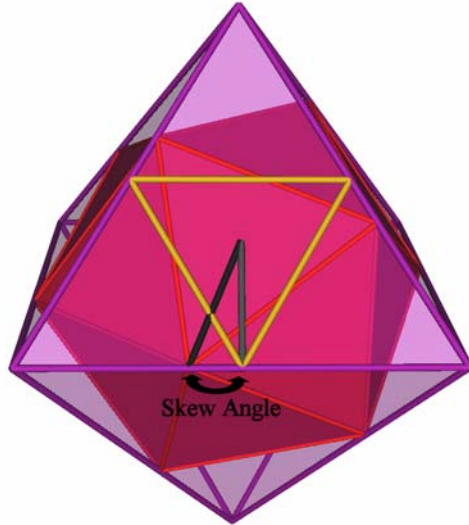
Figure 6 Defining the Skew Angle.
