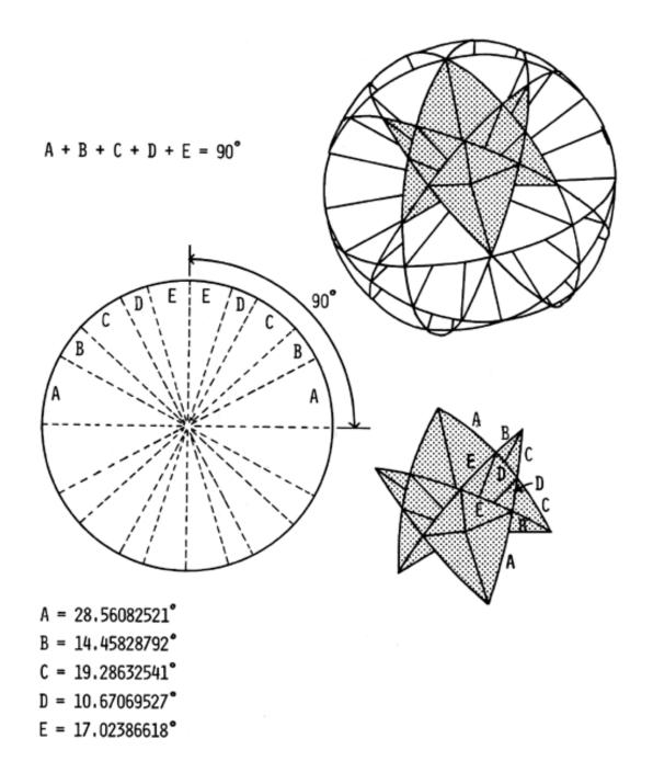
Fig. 450.10 The 12 Great Circles of the Vector Equilibrium Constructed from 12 Folded Units (Shwon as Shaded).
