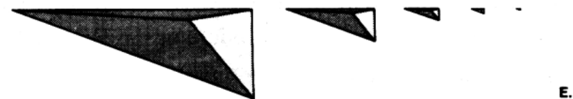
Fig. 986.561 T and E Modules: Minimod Nestabilities: Ratios of Angles and Edges: The top face remains open: the triangular lid will not close, but may be broken off and folded into smaller successive minimod tetra without limit.
